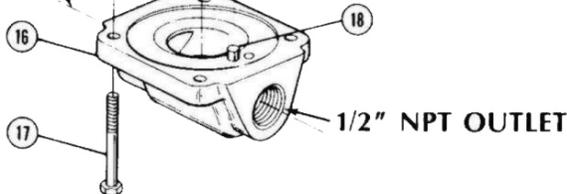
⬡\* Denotes assembly sequence numbers imprinted on part. Note that the plastic parts and rubber diaphragm are notched for proper assembly.
